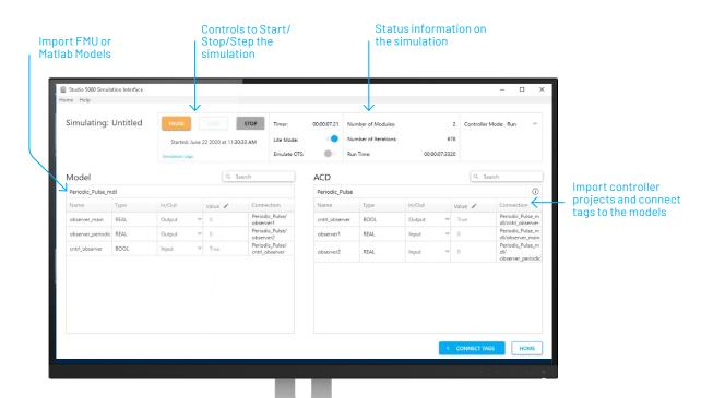
Start in a model, either MATLAB directly, or with a modeling software that uses the FMI standard
