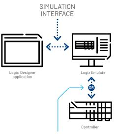
Download to either an emulated controller with Logix Emulate or a physical controller, such as ControlLogix® or CompactLogix™
