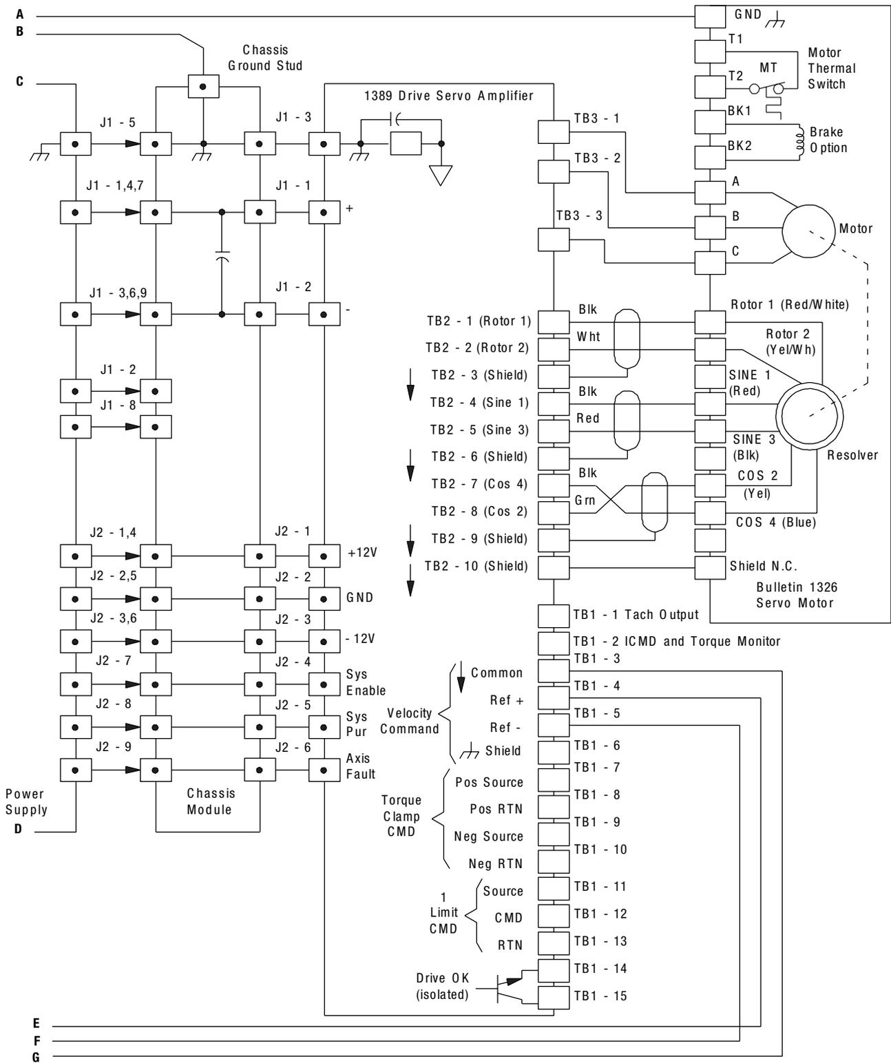
Figure 5.19 Wiring Diagram for 1391 Drives
