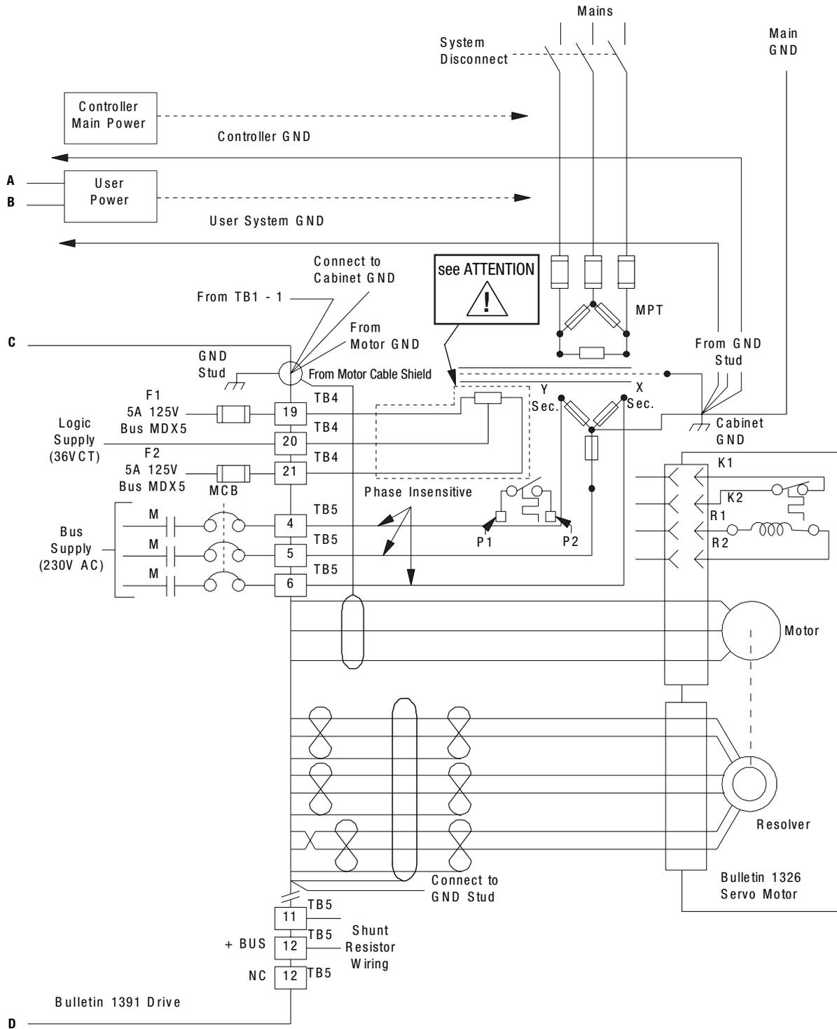
Figure 5.21 Wiring Diagram for 1392 Drives
