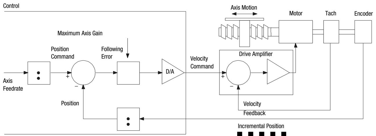
**Figure 7.5 Servo Loop Parameters in a Velocity Feedforward Loop**
