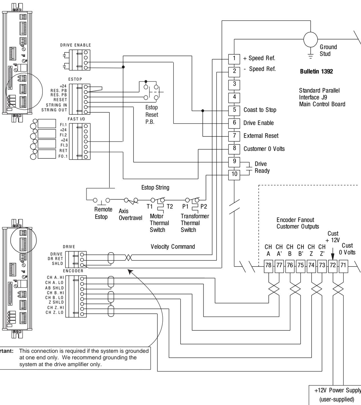
Figure 5.22 Wiring Diagram for 1394 Systems
