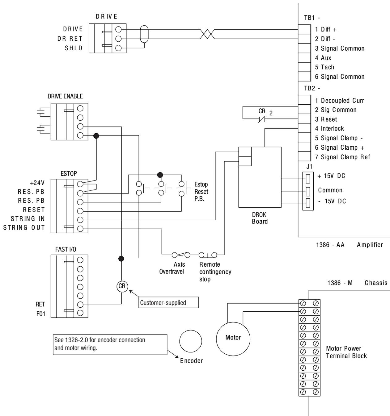
Figure 5.16 Wiring Diagram for 1388 Drives
