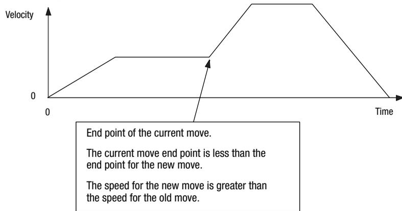
**Figure 8.12 Speed Increases, Direction Opposite, End Point Less**
