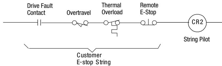
To wire Estop connections, refer to wiring diagrams for the drive you are using. The wiring of six different Allen-Bradley compatible drives is shown in the table below.
