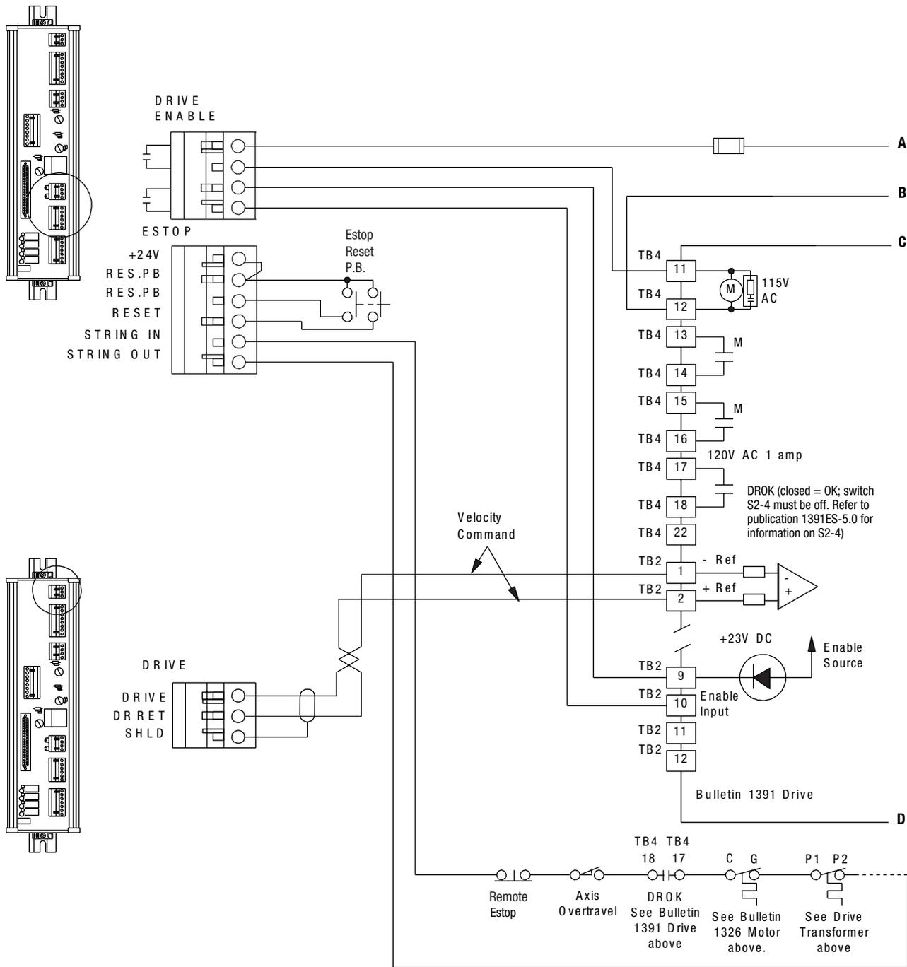
Figure 5.20 Wiring Diagram for 1391 Drives (continued)
