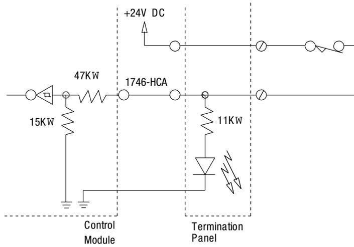
**Figure 5.3 Equivalent Fast Output Circuit**
