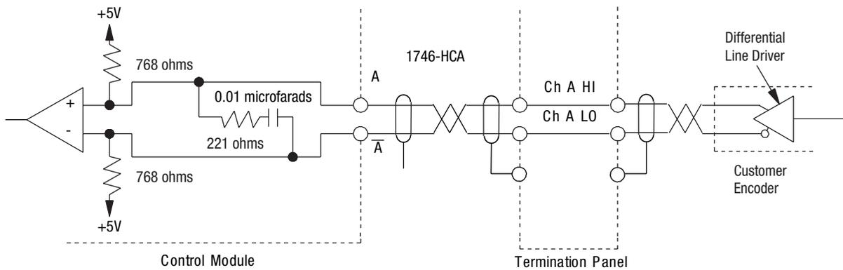
To operate the encoder, wire the encoder so that marker Z is true at the same time that A and B channels are true. To wire the encoder for consistent homing of the axis, do the following:
