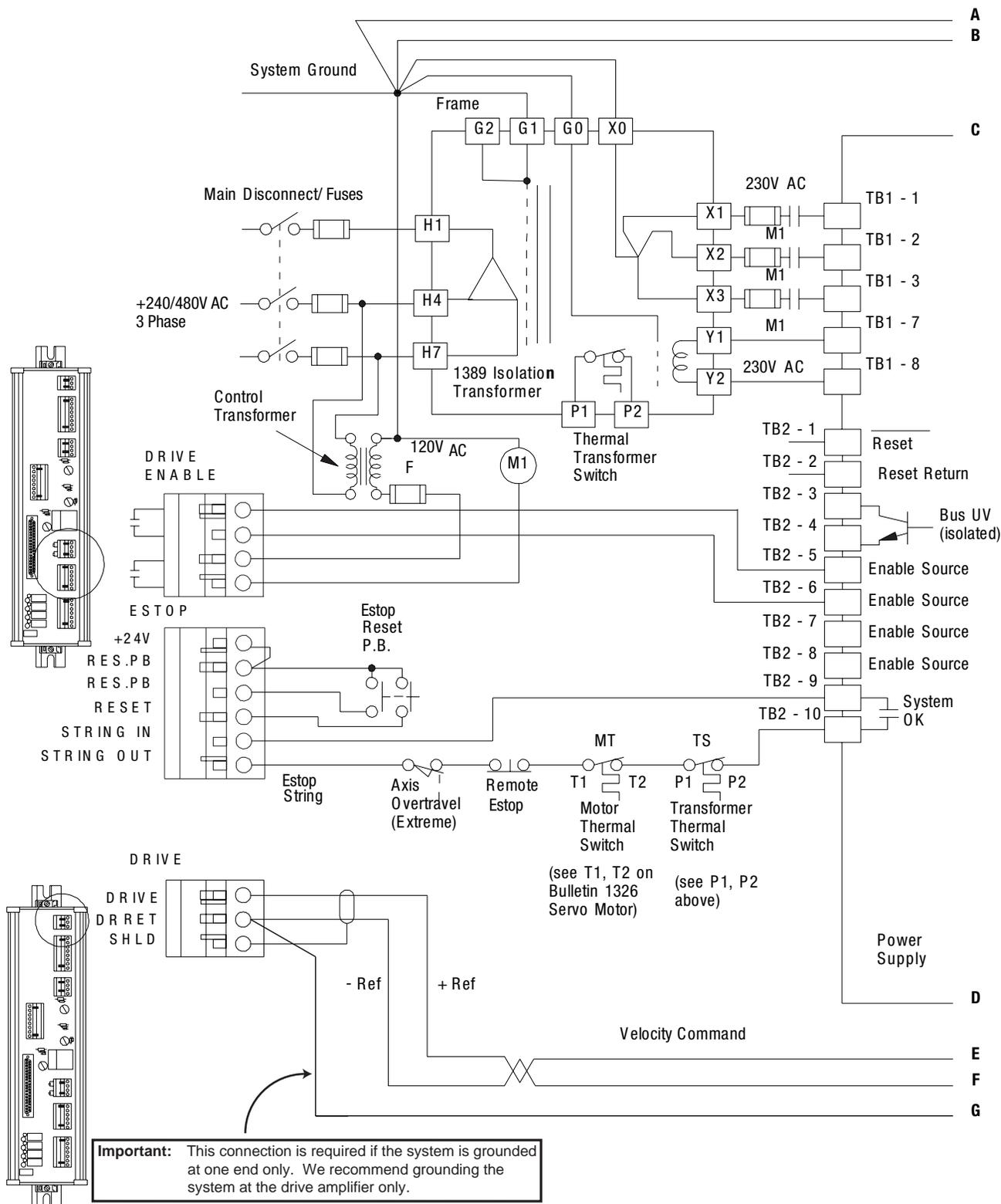
Figure 5.18 Wiring Diagram for 1389 Drives (continued)
