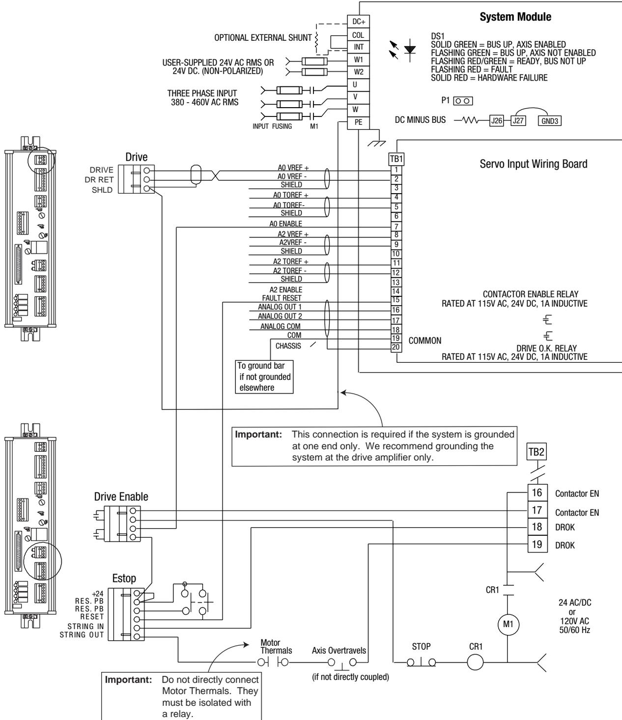
Figure 5.23 Wiring Diagram for 1394 Systems (continued)
