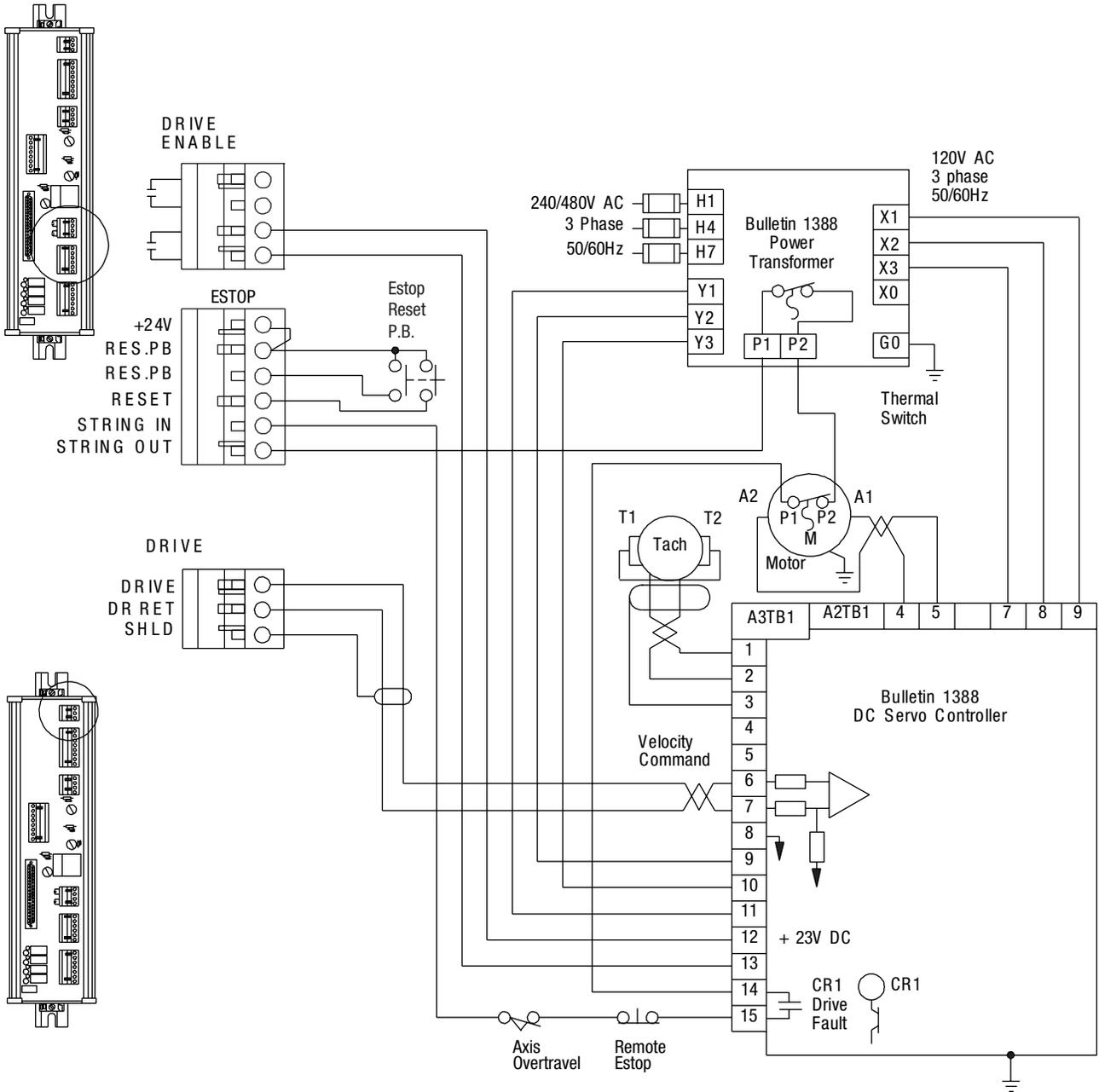
Figure 5.17 Wiring Diagram for 1389 Drives
