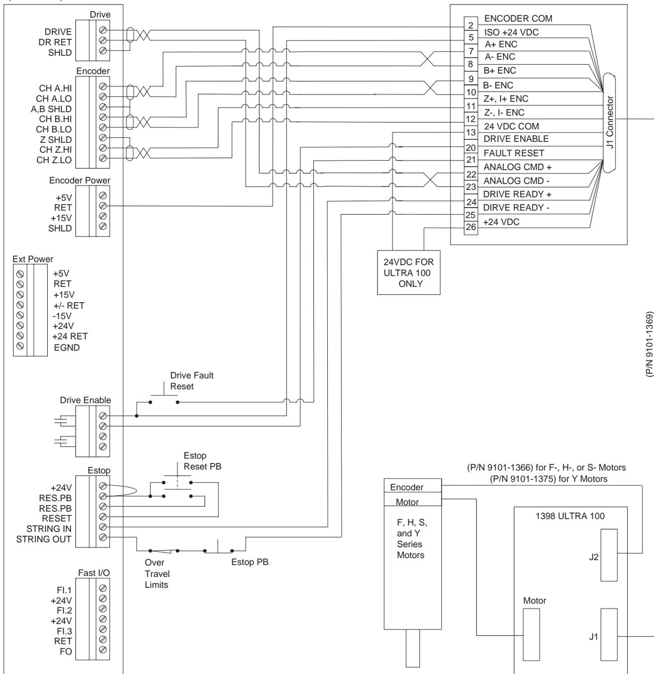
**Figure 5.25 Wiring Diagram for F, H, and S series ULTRA 100/200 When Homing to a Marker**
