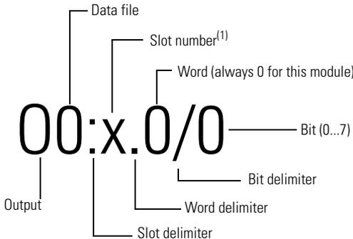
(1) I/O located on the controller (embedded I/O) is slot 0. I/O added to the controller (expansion I/O) begins with slot 1.
