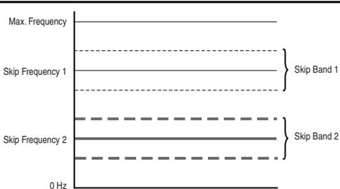
If skip bands overlap or touch, the center frequency is recalculated based on the highest and lowest band values.
