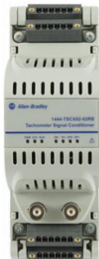
The Dynamix 1444 series tachometer signal conditioner expansion module is a two-channel monitor that converts the signal from common speed sensing transducers into a once-per-rev TTL class signal suitable for use by 1444-DYN04-01RA dynamic measurement modules.
