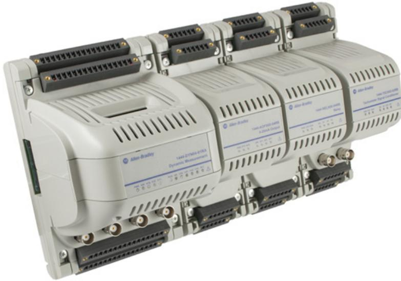
The system can measure dynamic signals such as vibration, strain or pressure, and position measures such as thrust, differential expansion, or rod position. Measurements are made in real time to protect industrial machinery from imminent failure, and/or, are further processed to calculate critical fault indicating parameters that can be used to assess the machines current and predicted health.
