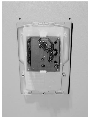
7. Insert the Panel Platform in the hole.
