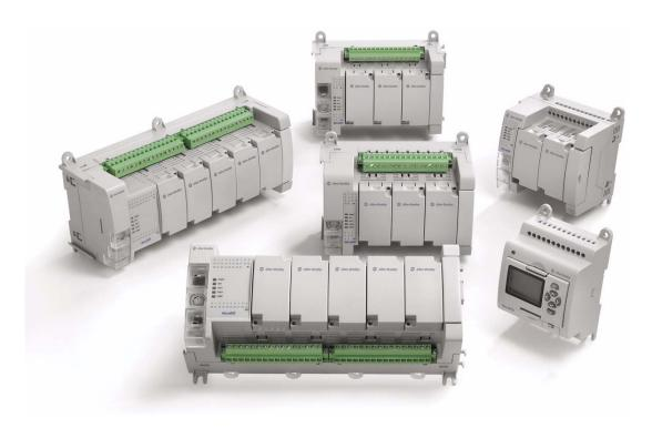
The Micro830 controller allows integration of as many as five plug-in modules. The plug-in modules enable machine builders to personalize the controllers to increase functionality. Most models offer removable terminal blocks and simplified communication via serial port.
