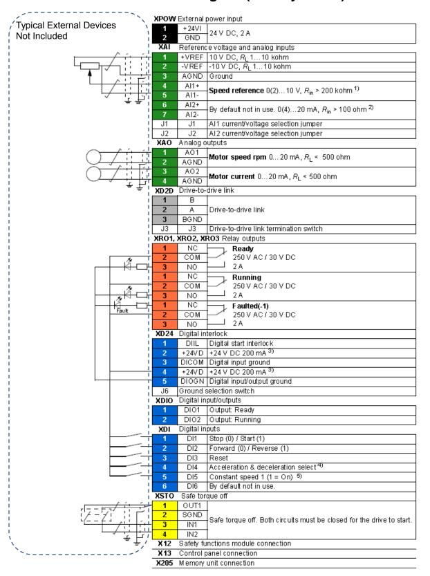
Control unit terminal wire sizes: 0.5 ... 2.5 mm<sup>2</sup> (24...12 AWG). Tightening torques: 0.5 N·m (5 lbf·in) for both stranded and solid wiring
