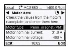
The ACS880 control panel features a set-up assistant that prompts the user through the commissioning process. It navigates thorough the parameters that pertain to initial set up and allows easy entry of motor and line settings. It then allows the selection of different ID run procedures, including normal rotation, reduced rotation, and without rotation, and to customize selections based on the existing conditions.
