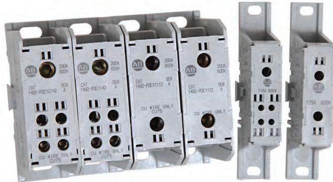
1492-PDME/PDE Enclosed Power Distribution Terminal Blocks are designed to prevent accidental contact with live connectors—without the use of additional barriers or shields. These panel mount devices have a compact footprint, and are available with either aluminum or copper terminals. Captive termination screws ensure that parts never get lost and the rugged thermoplastic housing will resist physical damage.
