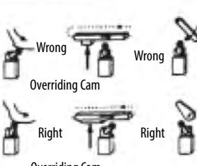
Cam or dog arrangements should be such that the actuator is not suddenly released to snap back freely.
