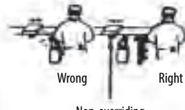
Limit switches should be mounted in locations which would prevent false operation by normal movements of operator or machine components.
