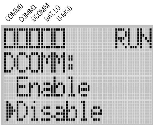
The DCOMM status indicator, which is the third of the five indicators at the top left of the LED display, is displayed in empty rectangle. It means that the communication configuration is set to a user-defined communication mode at present.
