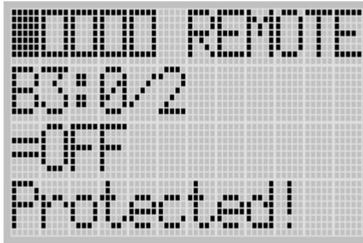
9. Try to move the cursor to the data value position by pressing the OK key. Because the B3:0/2 bit is a protected bit, you will find that the cursor does not move to the data value position.
