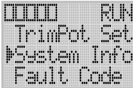
3. If System Info is selected, press the OK key. If not, select System Info using the Up and Down keys, and then press the OK key.
