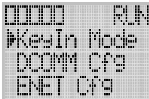
3. Select KeyIn Mode using the Up and Down keys, and then press the OK key.
