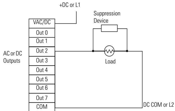
If the outputs are DC, we recommend that you use a 1N4004 diode for surge suppression, as shown below. For inductive DC load devices, a diode is suitable. A 1N4004 diode is acceptable for most applications. A surge
