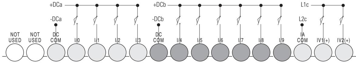
**1763-L16BBB and 1763-L16DWD Sourcing Input Wiring Diagram**
