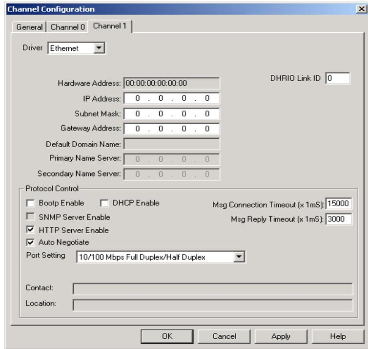
See the table below to configure the subnet mask and gateway address fields for each controller via your programming software.
