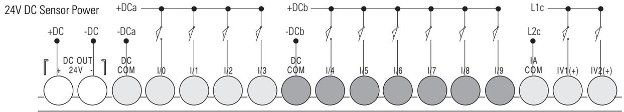
**1763-L16BWA Sourcing Input Wiring Diagram**
