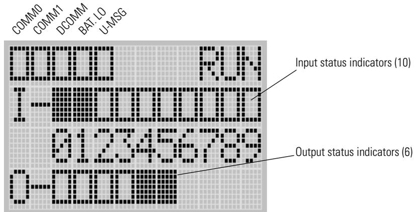
A solid rectangle is displayed when the input or output is energized. An empty rectangle is displayed when the input or output is not energized.
