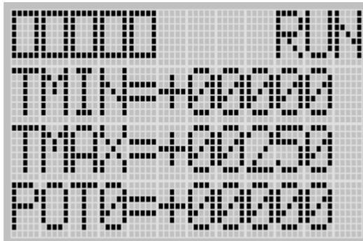
TMIN and TMAX indicate the range of data value for the trim pots, both POT0 and POT1. The factory default for TMIN, TMAX, and POT0 values are 0, 250, and 0 in decimal, respectively. TMIN and TMAX on this screen are read only, but you can change them using the LCD Function File in your application program. The TMIN and TMAX elements can only be changed by a program download.
