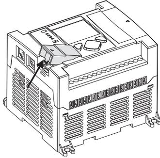
2. Align the connector on the memory module with the connector pins on the controller.
