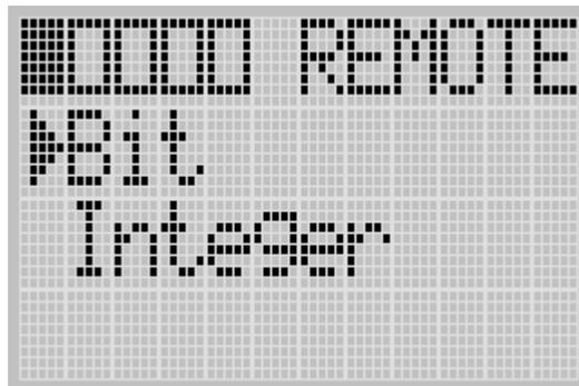
3. If Bit is selected, as shown in [step 2](#), press the OK key. If not selected, press the Up or Down key to select it and then press the OK key.
