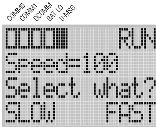
3. Hold down the ESC key **more than 3 seconds** to return to the Main Menu screen, as shown below.
