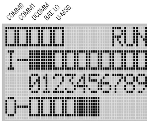
This is the default screen of the display, allowing you to monitor controller and I/O Status. For more information on the I/O Status screen, [see I/O Status on page 5-107](#).
