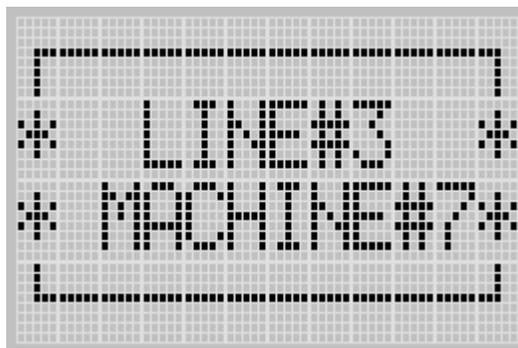
For more information on how to create and use a customized Startup screen, refer to the LCD Function File described in the MicroLogix 1100 Programmable Controllers Instruction Set Reference Manual, publication 1763-RM001.
