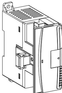
1762 Expansion I/O Connected to MicroLogix 1100 Controller
