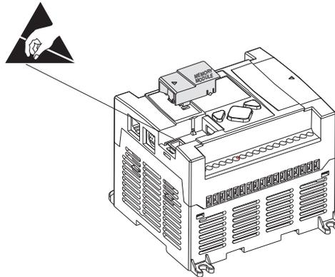
3. Firmly seat the memory module into the controller.
