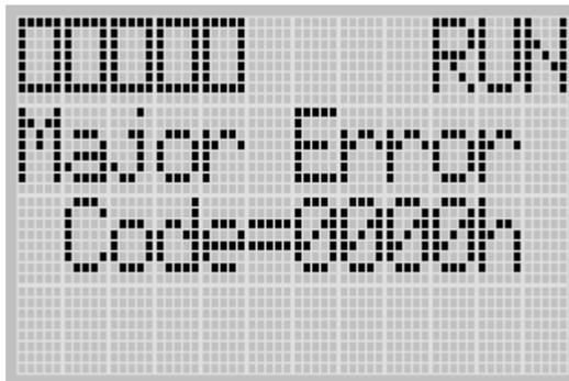
If a fault is occurred, its fault code is displayed, as shown below.
