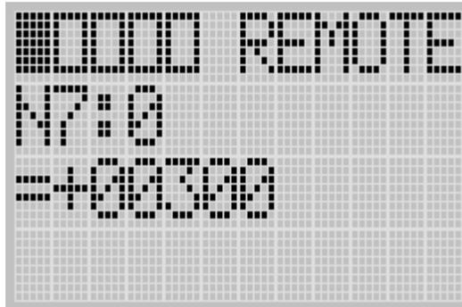
7. Press the Left key once. Then, press the Up key once. The second digit will change to “1”. Note that “1” is still flashing, which means the cursor is still at the data value position.
