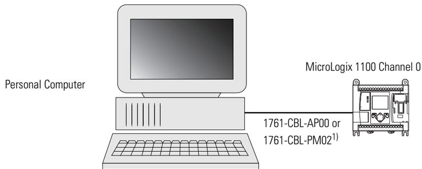
(1) Series C or later cables are required for Class I Div 2 applications.
