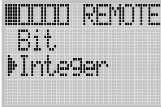
3. If Integer is selected, as shown in step 2, press the OK key. If not selected, press the Down key to select it and then press the OK key.
