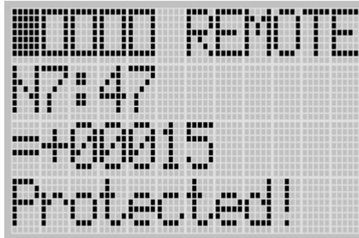
Press the Up key again, and you will find the target word does not change to “48”. It is because the maximum range of words you can monitor with the LCD is the first 48 words of the specified target integer file.
