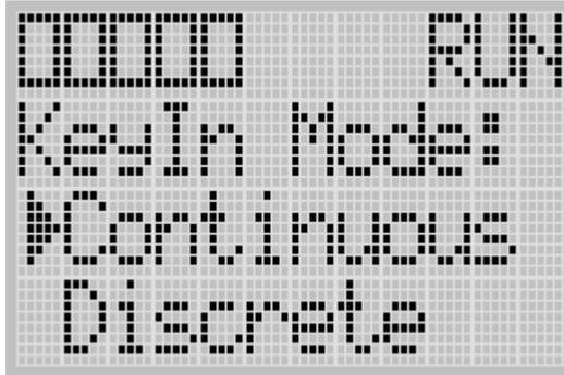
5. Press the Up or Down key to select the different mode, Discrete in this example, as shown below. Then, press the OK key.
