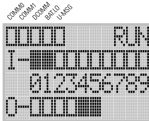
If the RTC battery is low and the controller is powered, the RTC operates normally. If the controller power is removed and the RTC battery is low, RTC data is lost.
