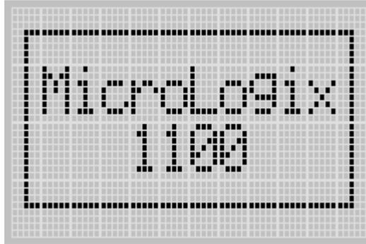
You can customize this Startup screen in your application program by defining a string data file that contains the string to display on the Startup screen and specifying the CBS element of the LCD Function File to the address of this string file.
