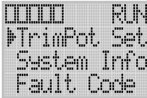
Trim pot data is updated continuously whenever the controller is powered-up.
