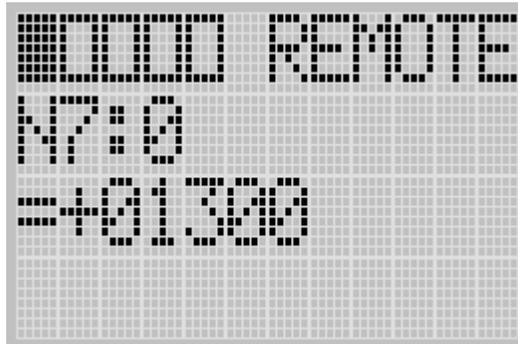
8. Press the Left key once. Then, press the Down key once. The sign digit will change to “-”, as shown below. Note that “-” is still flashing, which means the cursor is still at the data value position.
