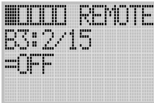
Press the Up key again, and you will find the target bit does not change to “3/0”. It is because the maximum range of bits you can monitor with the LCD is the first 48 bits (3 words) of the specified target bit file.
