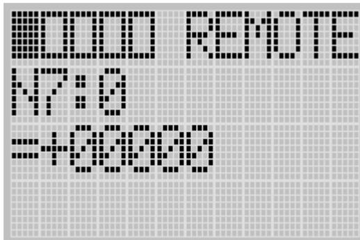
5. We will change the data value of the N7:0 word to the negative decimal value -1300. First, press OK to move the cursor to the data value position. Then, the last digit of “+00000” will be flashing, which means the cursor is at the data value position.
