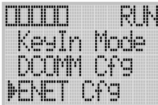
3. If ENET Cfg is selected, press the OK key. If not, select ENET Cfg using the Up and Down keys, and then press the OK key.
