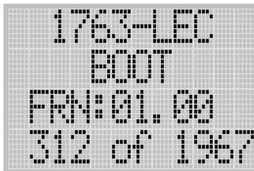
4. When the download is complete, the integrity of the new OS is checked. If the new OS is corrupt, the controller sends an error message to the download tool and flashes the Missing or Corrupt OS LED pattern. See [Missing/Corrupt OS LED Pattern](#) below.
