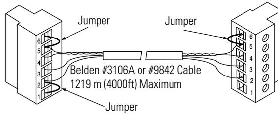
*MicroLogix 1100 Channel 0 to DH-485 Communication Cable Pinout*
