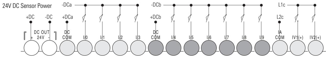
**1763-L16BBB and 1763-L16DWD Sinking Input Wiring Diagram**
