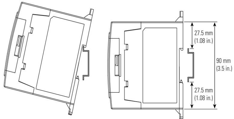
Follow this procedure to install your controller on the DIN rail.
