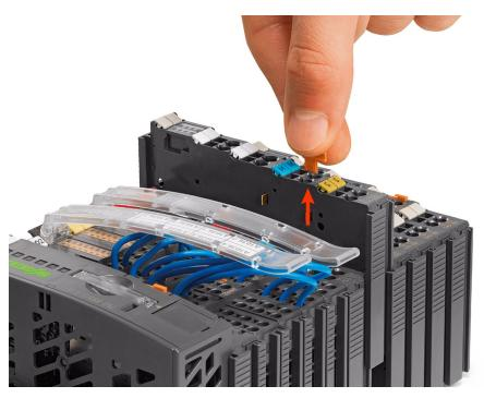
Figure 8: Removing the I/O Module (Example)
