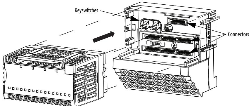
3. Press firmly and evenly to seat the module on the terminal base. The module is seated when the latching hooks are locked into the terminal base.
