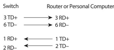
**Figure 6 - Four Twisted-pair Straight-through Cable Schematics**
