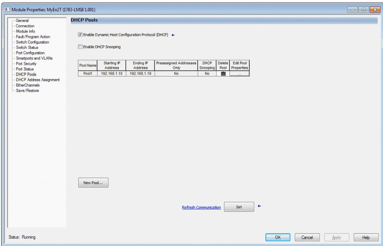
3. To enable DHCP snooping on the switch, click Enable DHCP Snooping.
