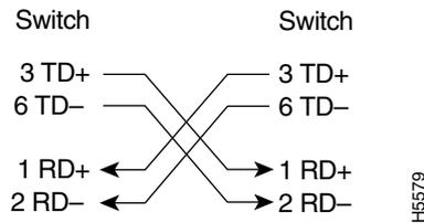
**Figure 8 - Four Twisted-pair Crossover Cable Schematics**
