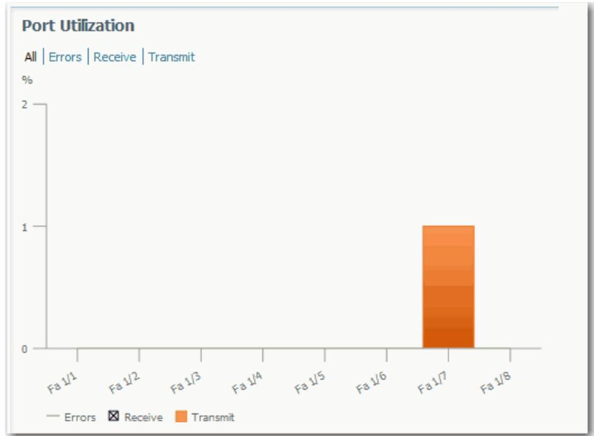
As you monitor the usage on the ports, note whether the percentage is what you expect during that given time of network activity. If usage is high when you expect it to be low, a problem can exist. Bandwidth allocation can also be based on whether the connection is operating in Half-duplex or Full-duplex mode.
