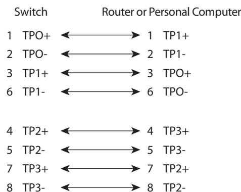
When connecting the ports to 10BASE-T- and 100BASE-TX-compatible devices, such as switches or repeaters, you can use a two or four twisted-pair, crossover cable.
