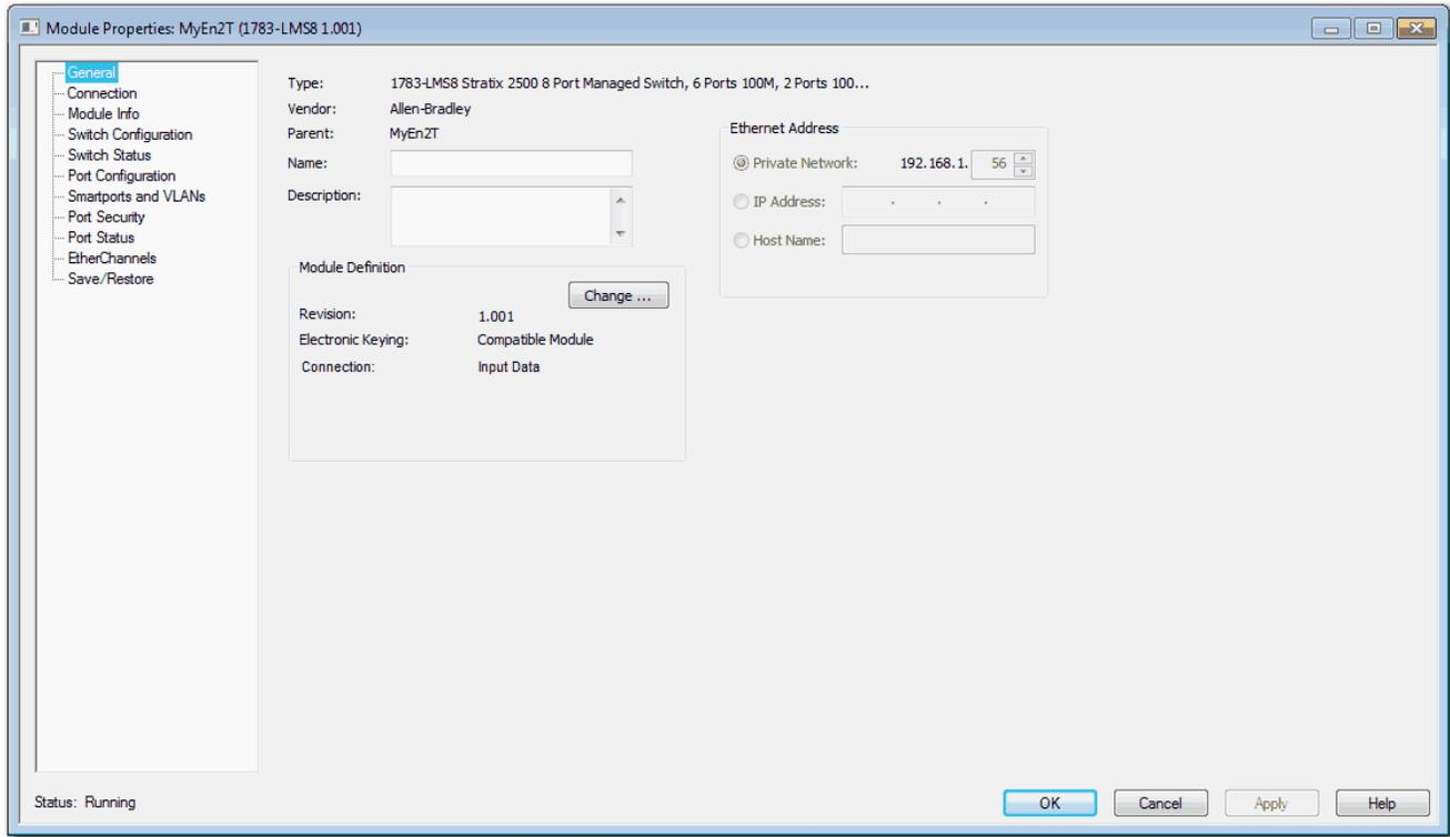
**IMPORTANT** The IP address and host name must match the values that you used during Express Setup. On the Module Properties dialog box, you can choose either an IP address or host name.
