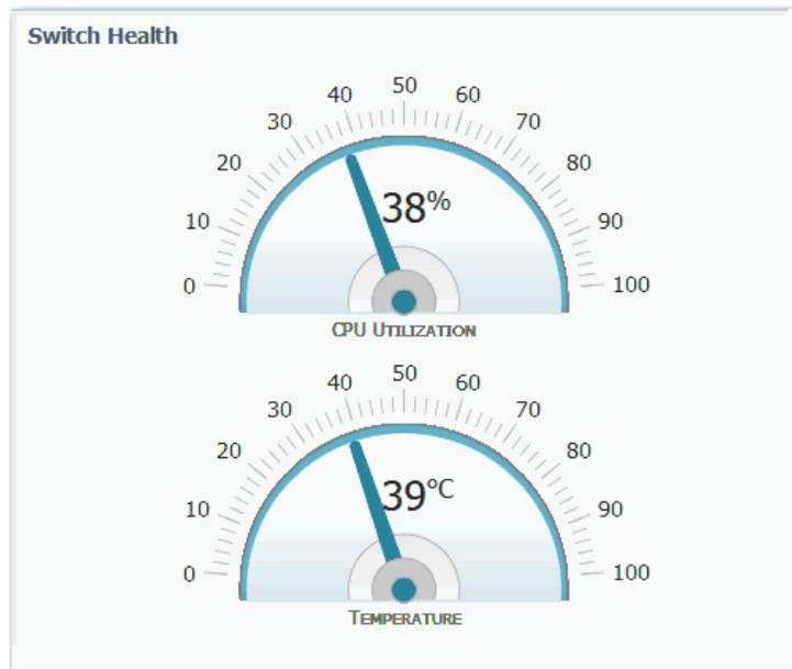
The CPU Utilization gauge shows the percentage of CPU processing power that is in use on the switch. Data is collected at each 60-second system refresh. The gauge changes as the switch experiences the network activity from devices sending data through the network. As network activity increases, so does contention between devices to send data through the network.
