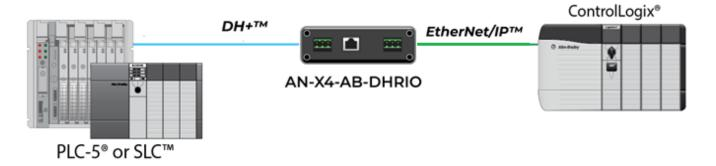
This operating mode helps the communication between an Ethernet-based processor with legacy processors on a DH+ network.
