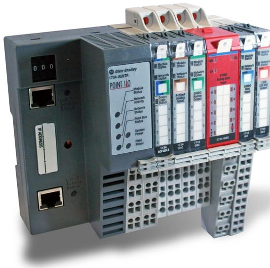
Each POINT I/O module mounts adjacent to the network adapter or another I/O module and removable terminal block (RTB) to connect all field-side wiring. The RTBs are part of the terminal base assembly. They are not included with the I/O modules and must be ordered separately.
