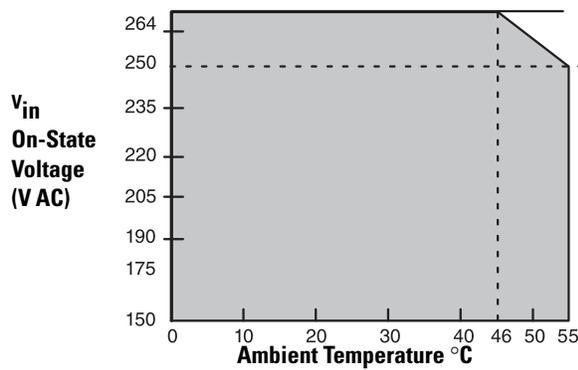
The area within the curve represents the safe operating range for the module under various conditions of user supplied 220V AC supply voltages and ambient temperatures.
