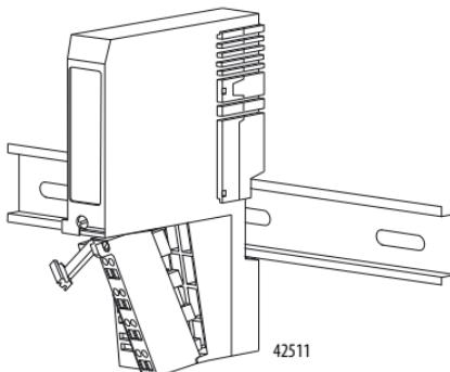
2. Remove the module to the right of the 1734-EP24DC or 1734-EP24DCK module from its base unit.
