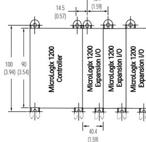
**NOTE:** All dimensions are in mm (inches). Hole spacing tolerance:  $\pm 0.4$  mm (0.016 in.).
