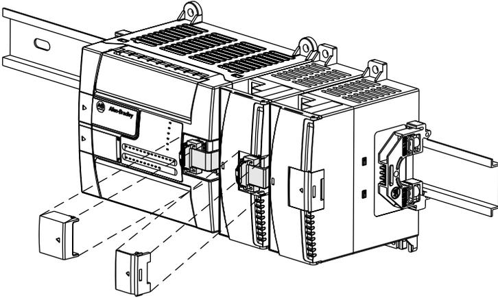
**Note:** Use the pull loop on the connector to disconnect modules. Do not pull on the ribbon cable.
