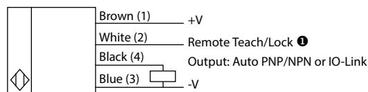
**① Normal operation:** No connection. Disabled in IO-Link operation.
