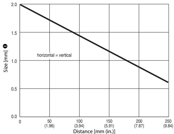
① The spot size is square in shape with one side dimension per the graph.
