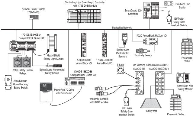
The above example network shows how almost any 24V DC safety-rated or standard sensor can be wired to any Guard I/O module to monitor the machine's status.
