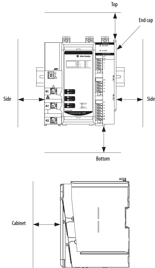
**IMPORTANT** CompactLogix 5380, Compact GuardLogix 5380, and CompactLogix 5480 systems can only be mounted horizontally.
