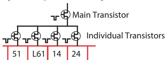
When pulse testing is configured (start with Logic Setting 0), the main transistor tests the outputs, which are then tested individually. The main transistor test pulse is 50  $\mu$ s wide. The pulse width on terminals 14 and 24 is 350  $\mu$ s wide, and the pulse width on terminals 51 and L61 is 200  $\mu$ s wide.
