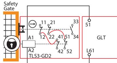
When using the TLS1, 2, or 3, the solenoid connections can be reversed, A1 can be connected to 51 or L61 and A2 can be connected to either 51 or L61.
