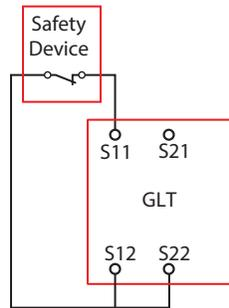
**Figure 9 - Connecting Mechanical Contacts of a Dual-channel E-stop**
