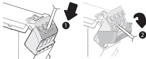
1. Insert the tip of a small screwdriver into the slot near the terminal screws.
