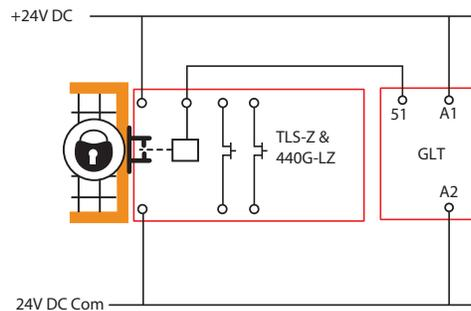
When connecting to the TLS-Z or 440G-LZ guard locking switch, the solenoid signal must be connected to terminal 51. Terminal L61 can also be used to drive a relay.
