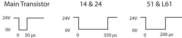
[Figure 27](#)...[Figure 29](#) show the pulse test pattern. This pattern depends on the GLT safety relay configuration and its state. [Figure 27](#) shows the pulse pattern for E-stop configurations. The pattern is repeated every 3750 ms.
