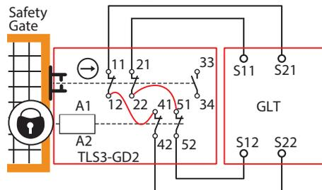
Since the TLS3-GD2 interlock switch has multiple contacts in series, the maximum safety performance rating is Cat 3 PLd and SIL CL2.
