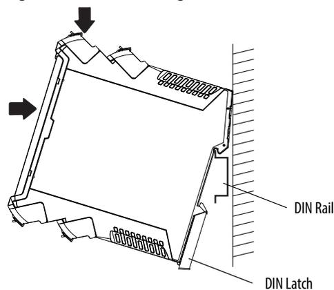
**Removal** - To remove the GLT safety relay, use a screwdriver to pry the DIN rail latch downwards until it is in the unlatched position. Then, swing the module up.
