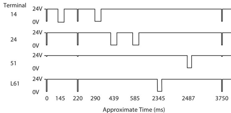
[Figure 28](#) shows the pulse test pattern on 51 and L61 when the GLT safety relay is configured as two high side outputs. The pattern is repeated every 2639 ms.
