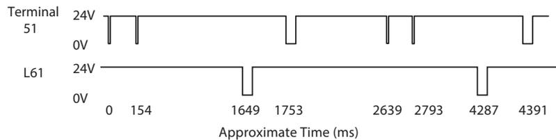
[Figure 29](#) shows the pulse test pattern on 51 and L61 when the GLT safety relay is configured as a high side/low side outputs. Terminal 51 is referenced to L61, not 24V common. The pattern is repeated every 2639 ms.
