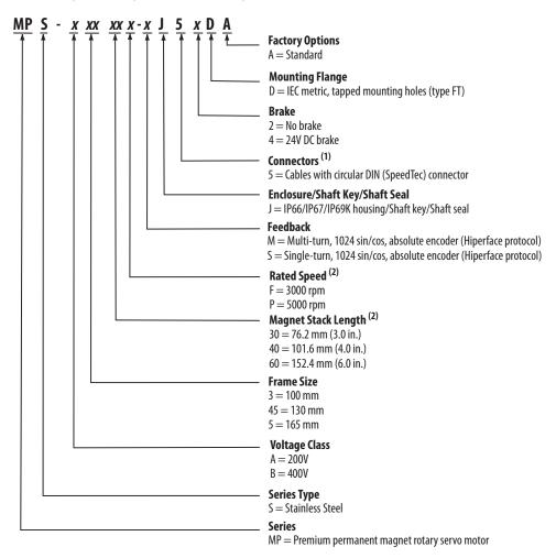
(1) The motor has 3 m (9.8 ft) cables with nickel-plated connector extensions.
