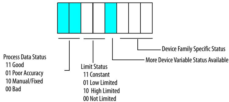
The Limit Status can be used to control windup in PID loops.
