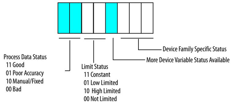
For example, if a valve positioner cannot open any further, it should set its HART.ChxSVStatus to 2#11100000 to indicate that the actual position value in the SV is Good (accurately measured) but is the subject of a High Limit. This status information can be used for windup control in PID loops and for other diagnostic purposes.
