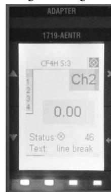
For digital modules, the screen displays diagnostic information in tabular form where the column labeled "C" indicates the channel number, "V" indicates the current value, "S" indicates channel status ( indicates "OK",  indicates "ERROR"), And "Message" Indicates the text message for diagnostic information.
