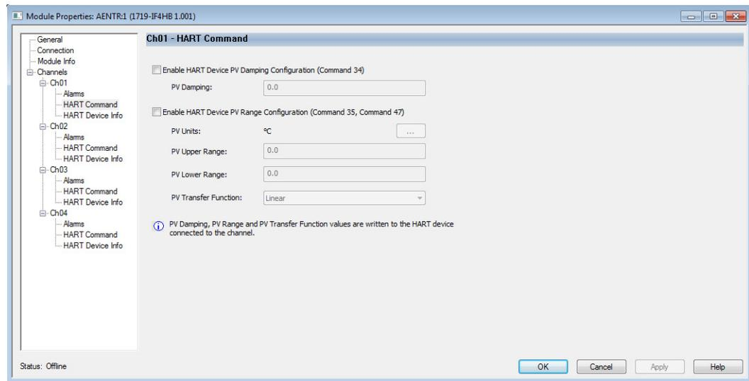
In the HART Command tab, you can specify HART device parameters for each channel. These values are sent to the HART device
