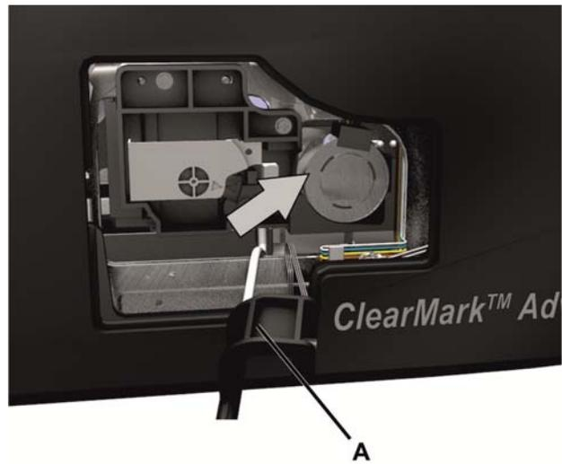
8. Slightly raise the injector (A) to remove it from the catch.
