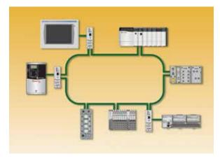
Dual-point adapters, coupled with the 1756-EN2TR supervisor-capable device, enable the use of Ring topology for greater system resilience.
