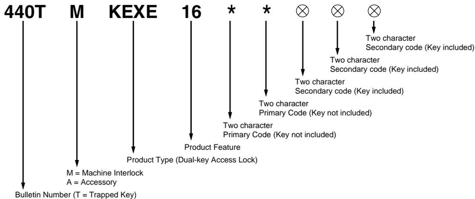
Order Cat. No. 440TMKEXE16AAABACACAC to get a key exchange unit with "AA" and "AB" primary codes and three "AC" secondary codes. The "AA" and "AB" keys are not included. The three "AC" keys, which are trapped in the secondary code barrels, are included.
