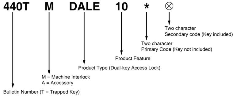
Order Cat. No. 440TMDALE100AAAB to get a Dual key Access Lock with an "AA" primary code and a "AB" secondary code, with a "AB" key included.
